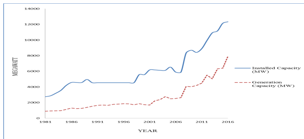
Figure 1: Installed capacity and actual generation capacity of hydroelectricity in Nigeria (1981 to 2018)
